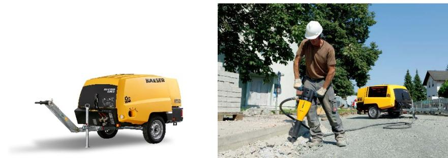
The "Mobilair 50" portable compressor from Kaeser combines sleek design with exceptional performance. The heart of this versatile 5m<sup>3</sup> class compressor hides beneath the corrosion- and scratch-resistant PE sound enclosure – now also available with a compressed air aftercooler.
