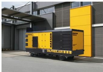
Portable powerhouse for air-hungry applications: Kaeser Kompressoren's new low-emission M 500-2 boasts a free air delivery range of quality dry compressed air from 38 m<sup>3</sup>/min (10.3 bar) to 45.8 m<sup>3</sup>/min (6.9 bar).
