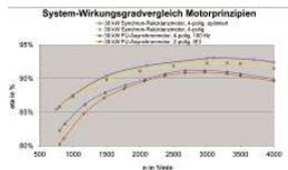
In comparison, the synchronous reluctance motor achieves significantly better efficiency values.
